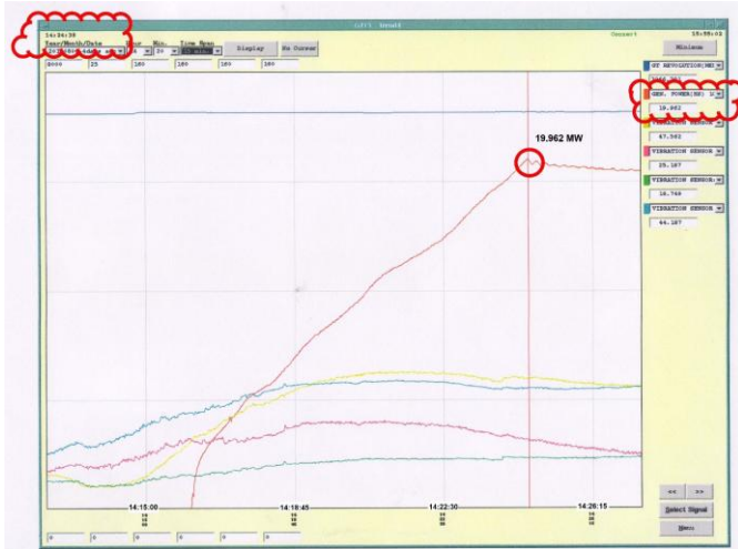
Fig. 5. power plant loading curve in base load
