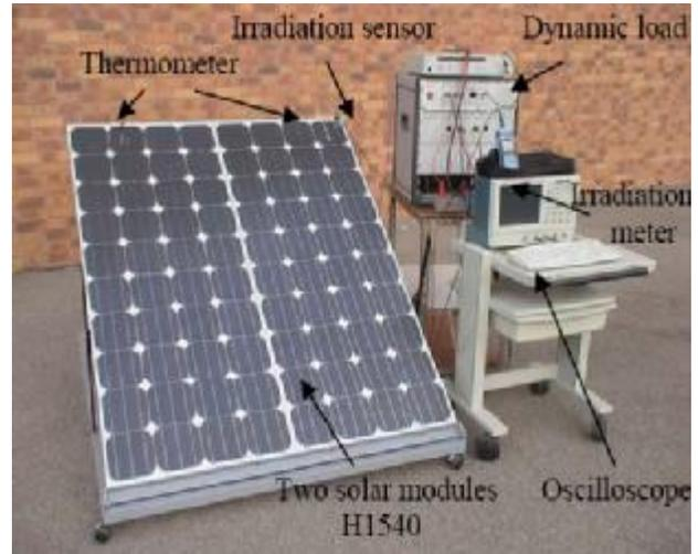
Fig.7-The test system for experimental results.
